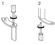
2. Fit the top handle bracket on the top left-hand side of the door (3) and screw the handle rod to the bottom handle bracket (4).
